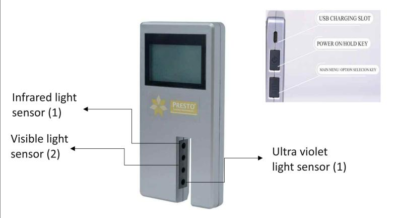
Transmittance Tester is used to check the amount of Ultra violet (UV), Visible and infrared (IR) light is passing through a sample. The readings will be displayed in percentage. Manufacturing processes can result in different transparency grades, impacting the durability and integrity of the sample's interior walls.
